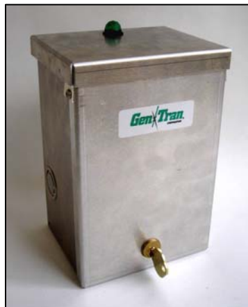
NEMA 3R aluminum enclosure includes hinged bottom and cover as well as a #2 keyed lock. Optional External Pilot Light (EPL) with 180° dome view shown on top.
