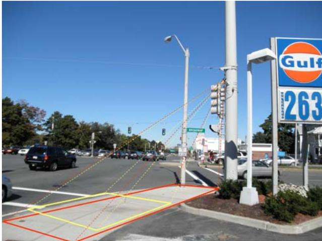
**MigmaIntersection™** is an outdoor passive pedestrian detector with interface to APS pushbuttons for automated locator tone triggering and pushbutton actuation. Using this detector, APS locator tone is silent unless pedestrians are within 12 ft from the signal pole. Based on the presence of pedestrians, APS or mechanical pushbuttons can also be automatically actuated.
