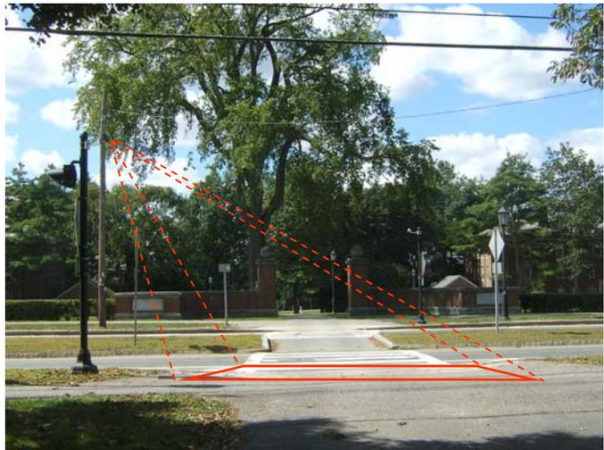
**MigmaMidblock™** is an outdoor passive pedestrian detector at the midblock crossings for automated beacon flasher actuation (flashing beacon) to alert the approaching vehicle drivers about the pedestrians who are about to enter the crosswalks.
