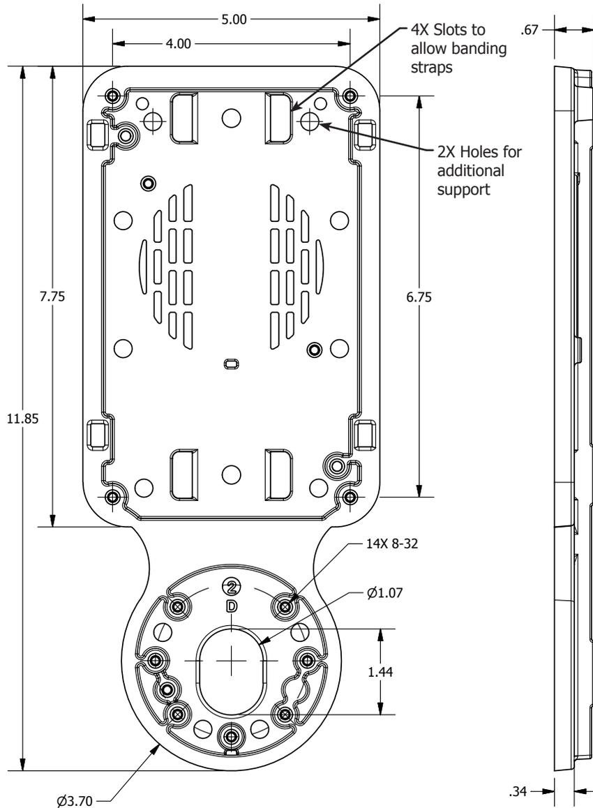
Polara's Push Button Frames are constructed to mount on a 2½" diameter pole up to a 24" diameter pole, or a flat surface. The cast aluminum structure and powder coated finish provides a low profile, very strong, and attractive mount for a pedestrian push button and sign.
